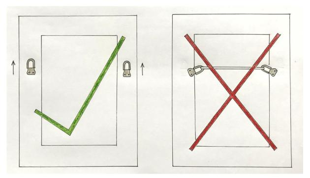
D-Rings should be attached vertically as shown above.
